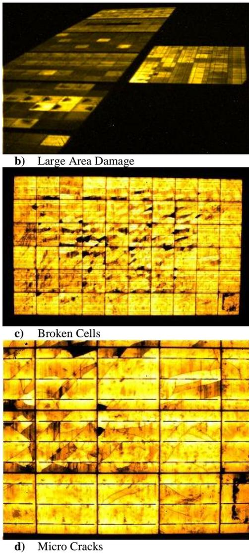
**Figure 2:** DaySy detects large area damage like PID, partially broken cells with inactive areas and damaged fingers from a distance. Close up images reveal micro cracks.
